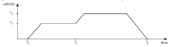
The CANopen Profile for Drives and Motion Control (DSP 402) refers to this method as the "set of set points" method.
