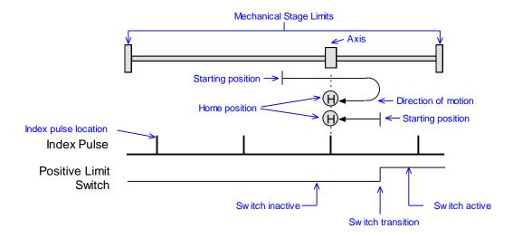
Note that in the homing method descriptions, negative motion is leftward and positive motion is rightward.
