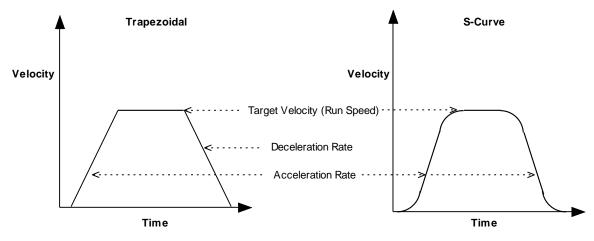
In a trapezoidal profile, jerk is unlimited at the corners of the profile (start of the move, when the target velocity is reached, when deceleration begins, and at the end of the move). S-curve profiling limits jerk or "smooths" the motion.
