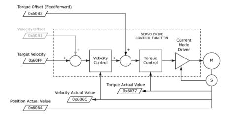
This diagram shows the CSV control function with real-time and other configuration parameters.
