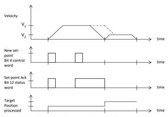
The dashed line in the first graph represents the velocity if the *change of set point bit* (bit 9 of the control word) is set.
