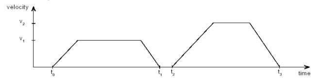
The CANopen Profile for Drives and Motion Control (DSP 402) refers to this method as the "single set point" method.
