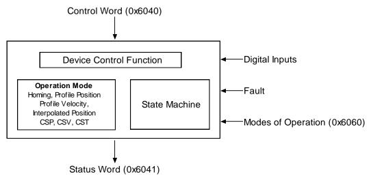
Other factors affecting control functions include: digital input signals, fault conditions, and settings in various dictionary objects.
