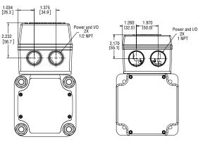
GSX30, GSX40<sup>°</sup> 'Applications with >20A rms will require the larger terminal box. GSX50, GSX60
