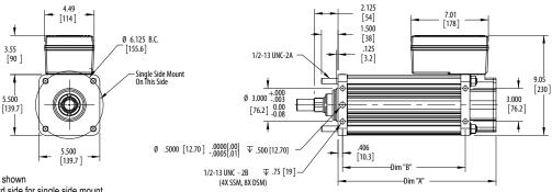
1. Three mounting styles shown 2. Shown view is standard side for single side mount
