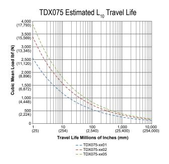
The L<sub>10</sub> expected life of a roller screw linear actuator is expressed as the linear travel distance that 90% of properly maintained roller screws are expected to meet or exceed. For higher than 90% reliability, the result should be multiplied by the following factors: 95% x 0.62; 96% x 0.53; 97% x 0.44; 98% x 0.33; 99% x 0.21. This is not a guarantee; these charts should be used for estimation purposes only.
