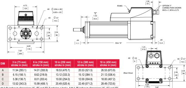
\* Add 1.61 inches to dimensions "A", "B" and "D" if ordering a brake. Add 1.78 inches to dimensions "A", "C" and "D" and dimension if ordering a splined  $\Delta$  main rod.
