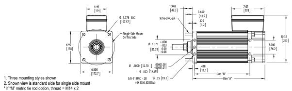
\* If "J" or "K" metric side mount options, M16 x 2.0  $\,$   $\pm$  16 mm with Ø 12 mm M7  $\pm$  12 mm Dowel Hole
