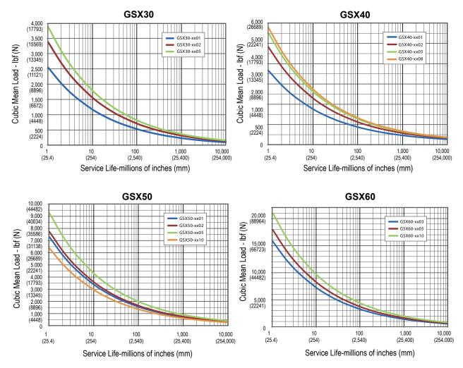
The L<sub>10</sub> expected life of a roller screw linear actuator is expressed as the linear travel distance that 90% of properly maintained roller screws manufactured are expected to meet or exceed. This is not a guarantee and these charts should be used for estimation purposes only.
