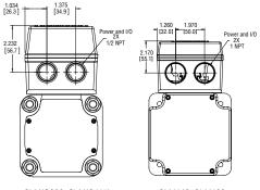
SLM/G090, SLM/G115<sup>•</sup> \*Applications with >20A rms will require the larger terminal box. SLM142, SLM180
