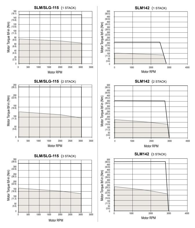
Test data derived using NEMA recommended aluminum heatsink 12" x 1/2" on SLM/SLG115 and 12" x 1/2" on SLM142 at 25°C ambient. For gearmotors, divide speed by gear ratio; multiply torque by gear ratio and effciency. Efficencies: 1 Stage = 0.91, 2 Stage = 0.86
