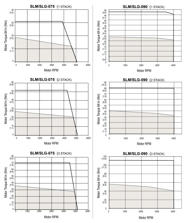
Test data derived using NEMA recommended aluminum heatsink 10" x 10" x 3/8" on SLM/SLG075 and 10" x 10" x 3/8" on SLM/SLG090 at 25° C ambient. For gearmotors, divide speed by gear ratio; multiply torque by gear ratio and effciency. Efficencies: 1 Stage = 0.91, 2 Stage = 0.86
