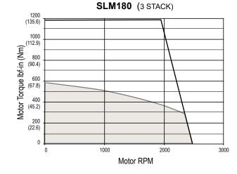
Test data derived using NEMA recommended aluminum heatsink 16" x 16" x 1" on SLM180 at 25°C ambient
