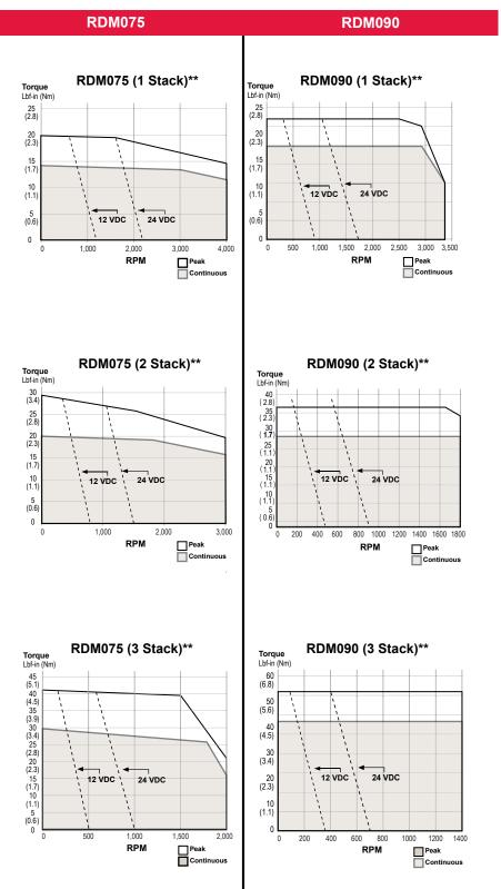
For RDG gearmotors, multiply torque by ratio and efficiency. Divide speed by gear ratio. \*\*RDM075 and RDM090 test data derived using NEMA recommended aluminum heatsink 10" x 10" x 3/8" at 40°C ambient
