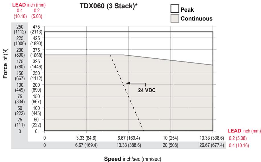
\*Test data derived using NEMA recommended aluminum heatsink 10" x 10" x 3/8" at 40°C ambient.
