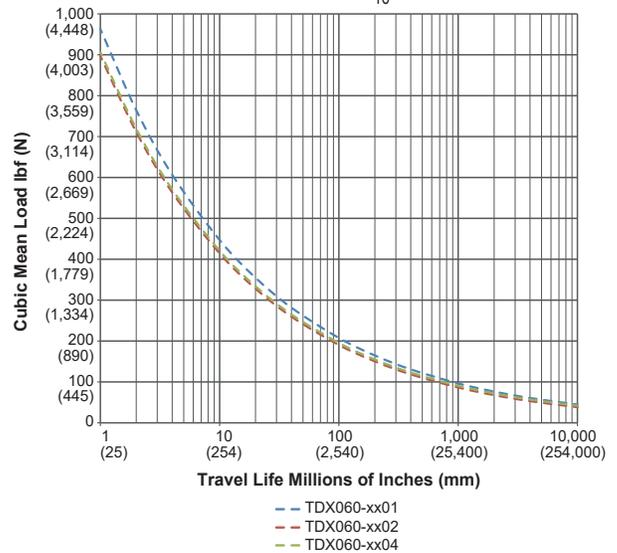
The  $L_{10}$  expected life of a roller screw linear actuator is expressed as the linear travel distance that 90% of properly maintained roller screws are expected to meet or exceed. For higher than 90% reliability, the result should be multiplied by the following factors: 95% x 0.62; 96% x 0.53; 97% x 0.44; 98% x 0.33; 99% x 0.21. This is not a guarantee; these charts should be used for estimation purposes only.
